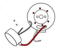
6- Remove the cable from the reel without turning the reel. Loosen the nuts that secure the outer wing of the reel.
