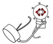
4- Loosen the fixing nuts of the brushes and remove the brushes by sliding them outwards.
